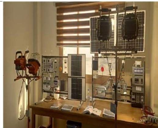
Example of generating electricity from small solar panels (Beni-Suef University - Faculty of Engineering, Beni-Suef)
